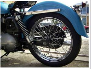
The left rear is clean on old K-models, no brake or sprocket in the way of those beautiful spokes. Note the "flip" on the end of the read fender, used on K's and early Sportsters.
