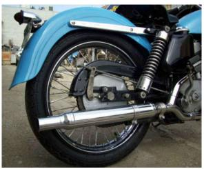
Stock tail light, although chromed, not black. Stock exhaust works well, its only 45 cubic inches, after all.
