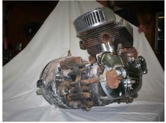
There are no visible welds on the back. I live near San Jose, where Kenny and Cary Puccio could fix any case problem, including big holes and missing chunks. The Sportster sprocket cover does not line up with the gearcase. A brake switch is missing that attaches to that boss on the back of the primary cover.
