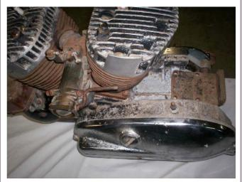
Even little things like that stud and nut on top of the case primary are a treasure. Its is likely the 1952 stud that came with the motor. the holes for the motor mount bolts go into the transmission, so there will be dirt in the tranny. Early K-models don't have a trap-door like Sportsters. You have to split the cases to work on the transmission.
