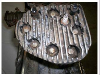
The rear head has the little bobbins that space off the top motor mount. With all the other chrome, I thought the heads had been chromed too. They are actually polished. The bolts are supposed to be cadmium plated, not chrome. Colony sells cad plated ones.
