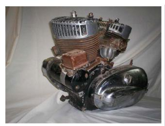
The front view shows the generator to be in good shape. The regulator looks too big for this year, I will have to do some research and see if it is the correct one for a '52. Amazing the oil pressure switch has not been broken off.
