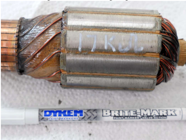
A Dykem paint pen notes the 17 k \Omega reading, it should be closer to 1 \Omega .
