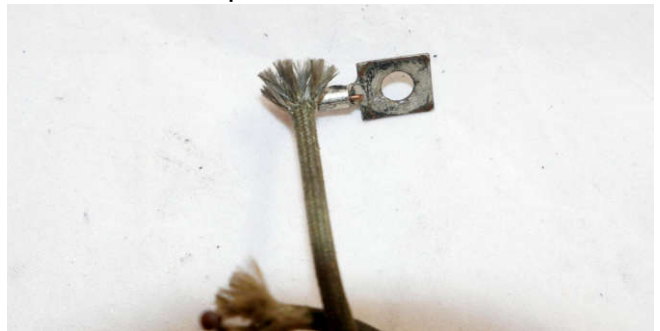
A field coil connection terminal.
