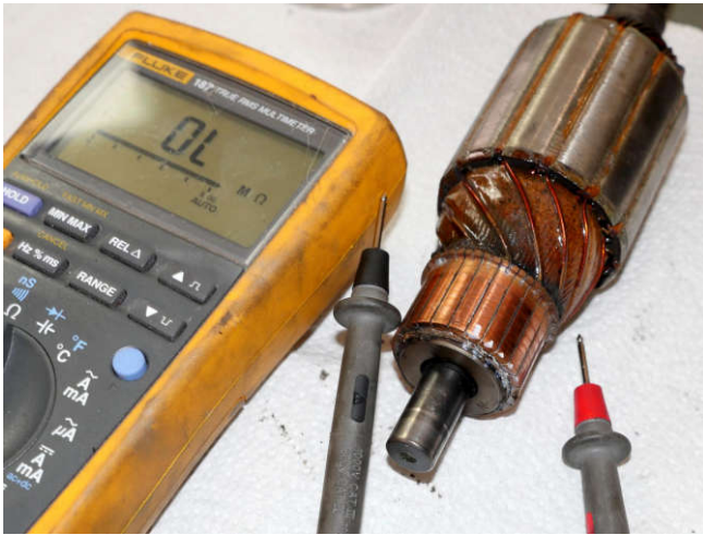
Measuring across the commutator found several segments reading high.
