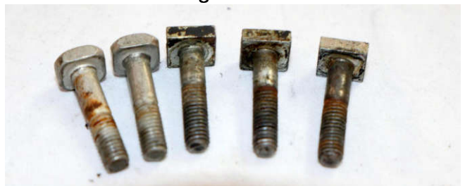
Aftermarket terminals have sharp corners that cut the paper washer. A bike with zero ohms field coil measurement might be cured with a new square paper washer. You can loosen the field terminal then tighten it without letting it spin and fix the generator without taking it off the bike.
