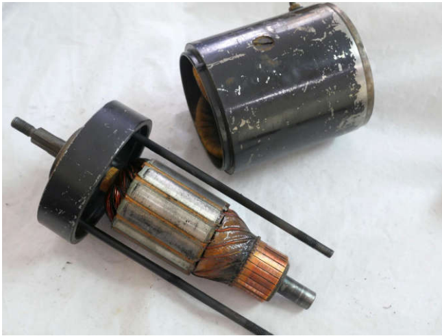
The frame separates from the drive-side end bell, which still holds the armature.
