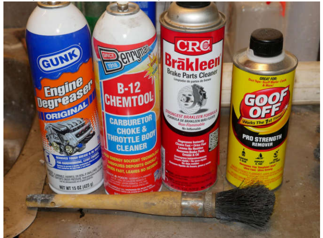
Engine degreaser is mild, but Chemtool, Brakleen, and Goof Off are strong. That brush is ideal to get into crevasses.
