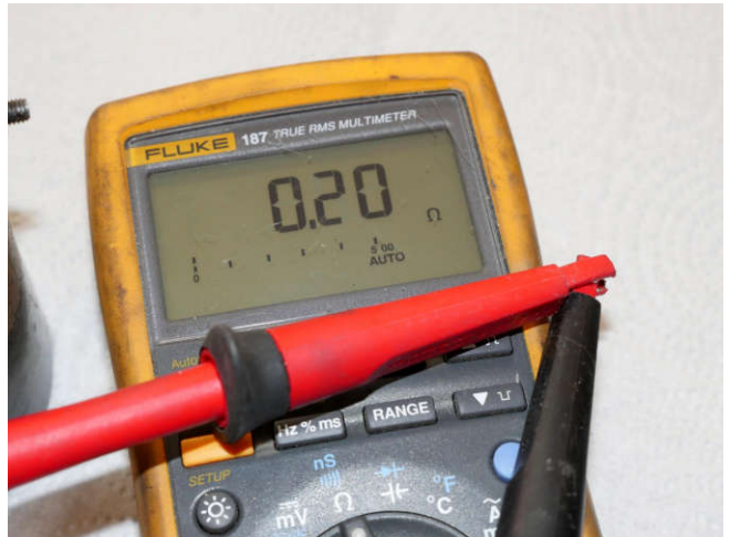
For such low resistance measurements, you can measure the leads and subtract.
