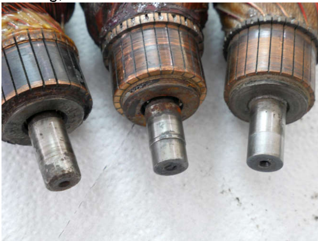
Armatures with ruined bearing surfaces. Left and middle are obviously bad, even smooth wear on right is unacceptable.
