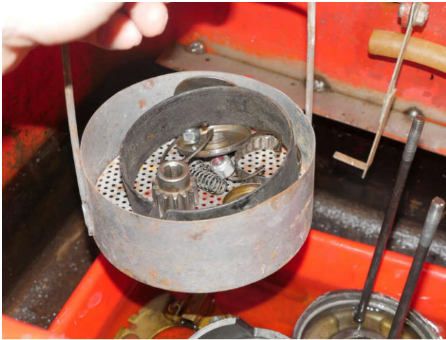
Small parts fit into a basket. No solvent on the brushes or bearings either.
