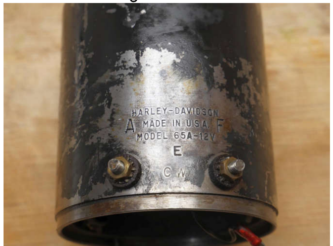
A shot of carb cleaner took the paint off the stamped label area. Wear gloves.
