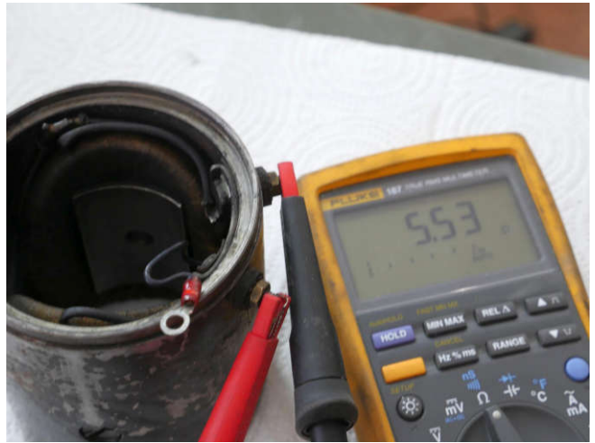
Recheck the field coil resistance. It should be between 5 \Omega and 6 \Omega for 12-volt units.
