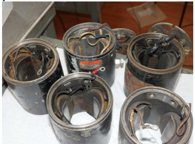
A collection of frames shows factory and aftermarket terminals and coils. The air gap between the armature is critical.
