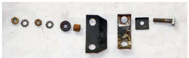
Over-torque on the field terminal will cut a corner into that black paper washer second from the right. This shorts the field.
