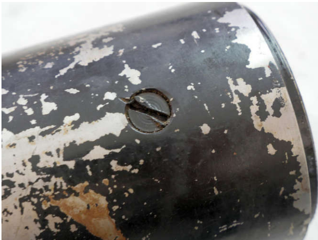
If the field coils are bad, you have to grind back this stake and impact out the screws.
