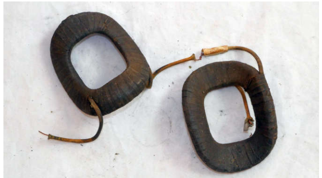
A pair of field coils, but with one missing a ring terminal. You can't solder this, it gets too hot. A crimp connection would work.
