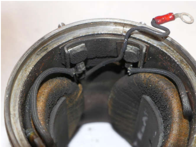
The left terminal has a field coil and the armature wire attached. The right terminal has the other end of the field coil.
