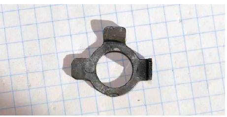
Sportster 34168-52 shifter cam lock tab. You use a new one every time, and bend the one of the little tabs against the bolt head to lock the bolt in place.
