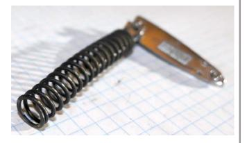
This view shows how the wear is worse on one end of the spring. If you are in the tranny, it might be a good idea to carefully inspect these springs and replace any that are worn flat anywhere.
