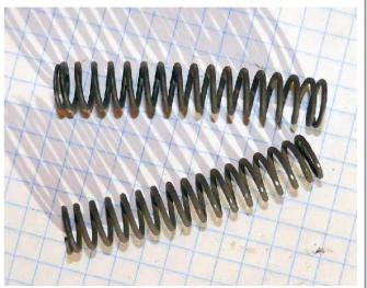
The springs tend to bendinto an arc from riding in the housing for years. This might be due to losing their temper, ot to the springs wearing in a certain way.
