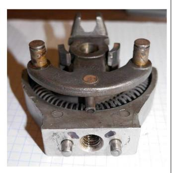
Here is the housing with the carrier partially installed. You can see how the spring stops are as wide as the pin in the carrier. This way the springs don't fight each other as they center the carrier and hence, the shifter lever.
