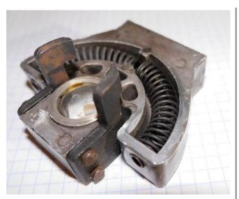
Here is a view of the two shifter support springs as installed in the housing. At rest, they press against those square features, they do not bear on the pin in the shifter carrier that they center.
