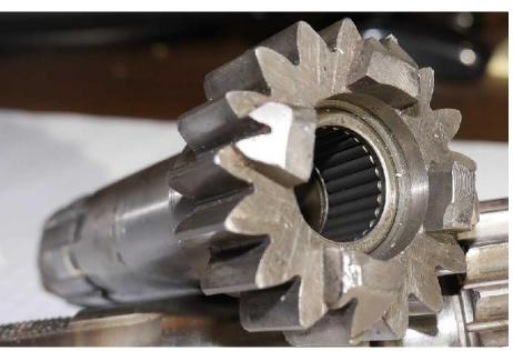
This Torrington needle bearing is pressed into the clutch gear. A thrust washer gets pressed in over it.
