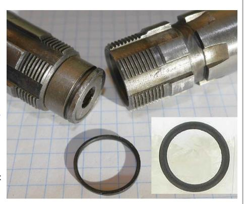
11103 on left, near the early model dry-clutch gear with the extentison pressed in. The 11119 is on the right. It is much bigger and goes in that wide groove in the electric start dry clutch gear above it.
